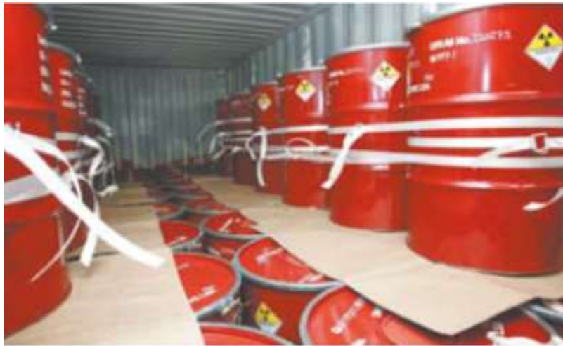
Figure 2: Drums secured safely within a GP container
