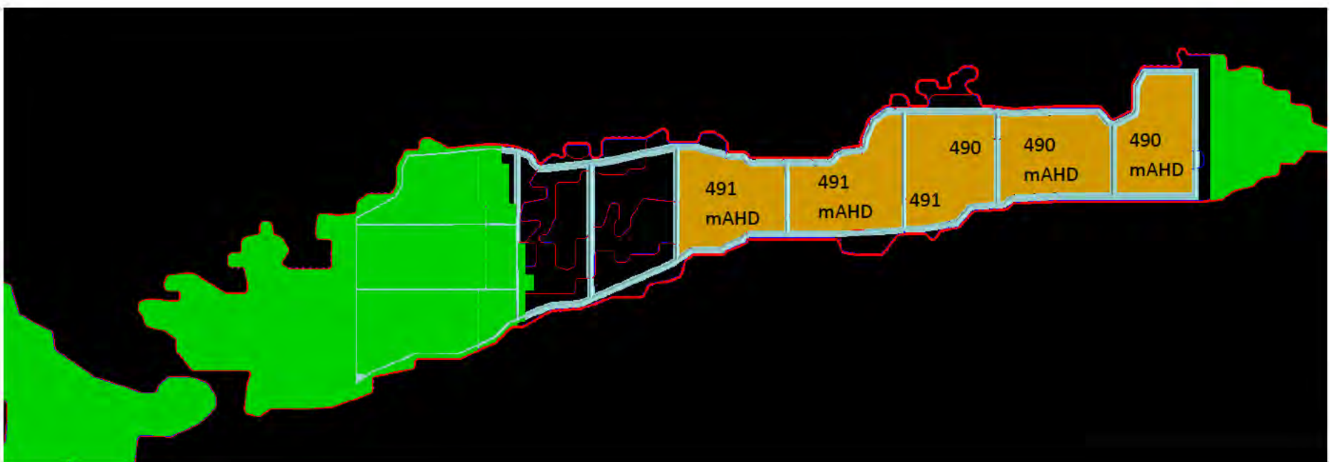
Figure 5.6e Sequence of mining, tailings deposition and mine pit backfilling at Year 5 (tailings deposition in its 3 rd year)
