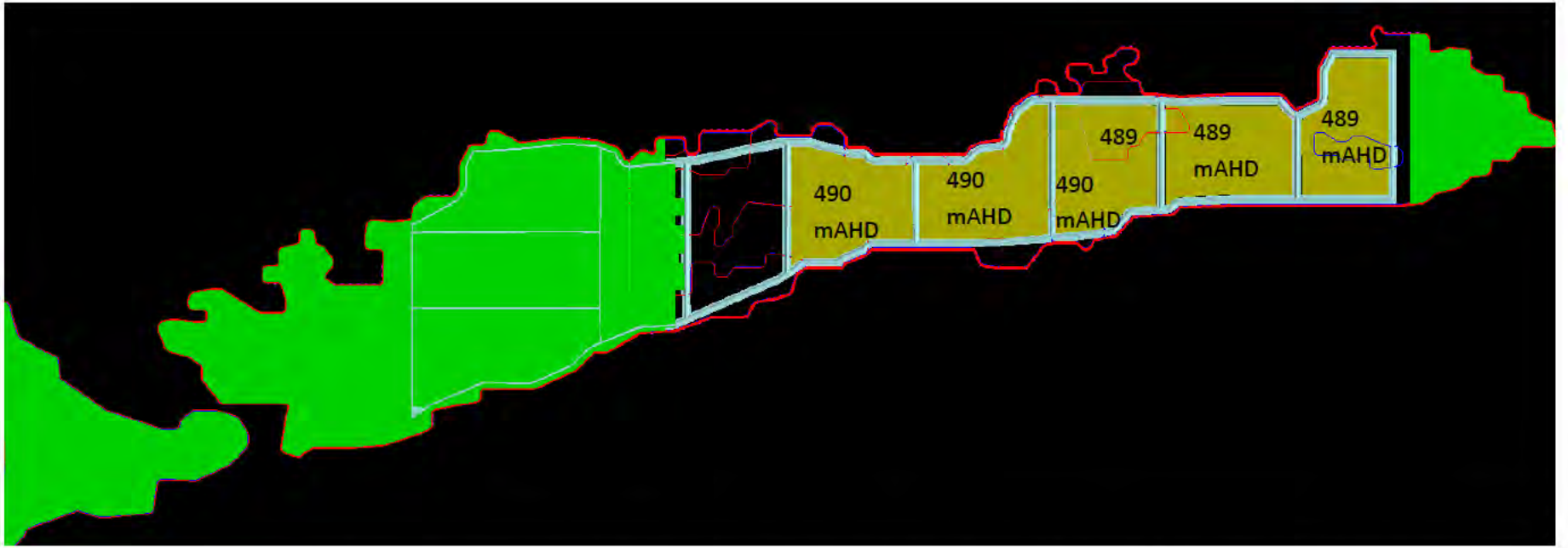
Figure 5.6d Sequence of mining, tailings deposition (in greenish yellow) and mine pit backfilling at year 4 (tailings deposition in its 2 nd year)
