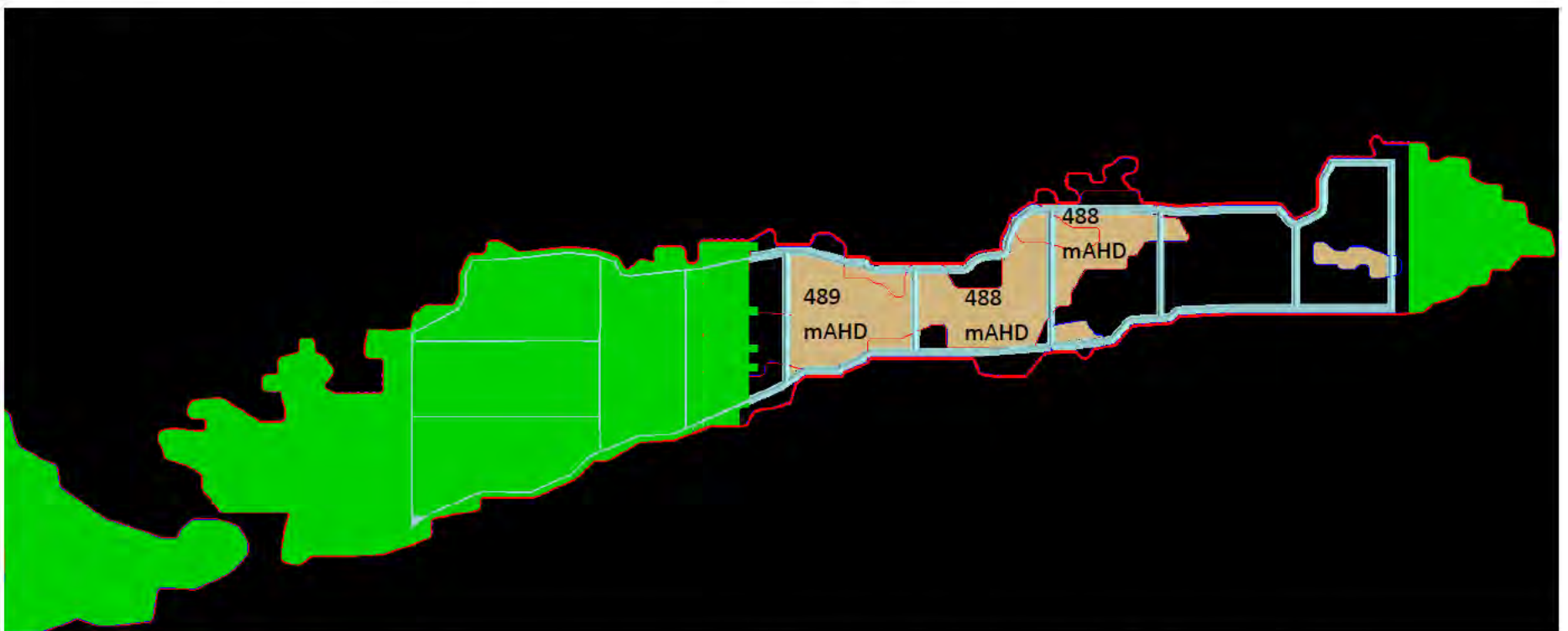
Figure 5.6c Sequence of mining, tailings deposition and mine pit backfilling at year 3 mining (year 3 is the first year of tailings deposited. Tailings in light brown.)
